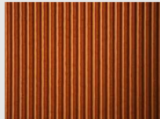
150µm Pitch / 50µm Pad L/S: 11/11µm, Before Cu seed layer etching
